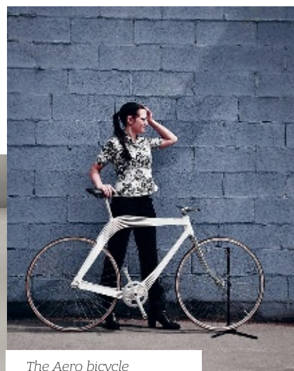
The Aero bicycle with lamellar wood frame, whose form is generated through the simulation of the forces typically applied to the vehicle. Concept and design: Martino Hutz (Martino Hutz Architecture). Development and engineering: Atanas Zhelev and Mariya Korolova (Digital Architects). Project done in collaboration with: University of the Applied Arts of Vienna/Institute of Architecture, Studio Zaha Hadid, Maveo.net, Altair Engineering, Hoeller.
