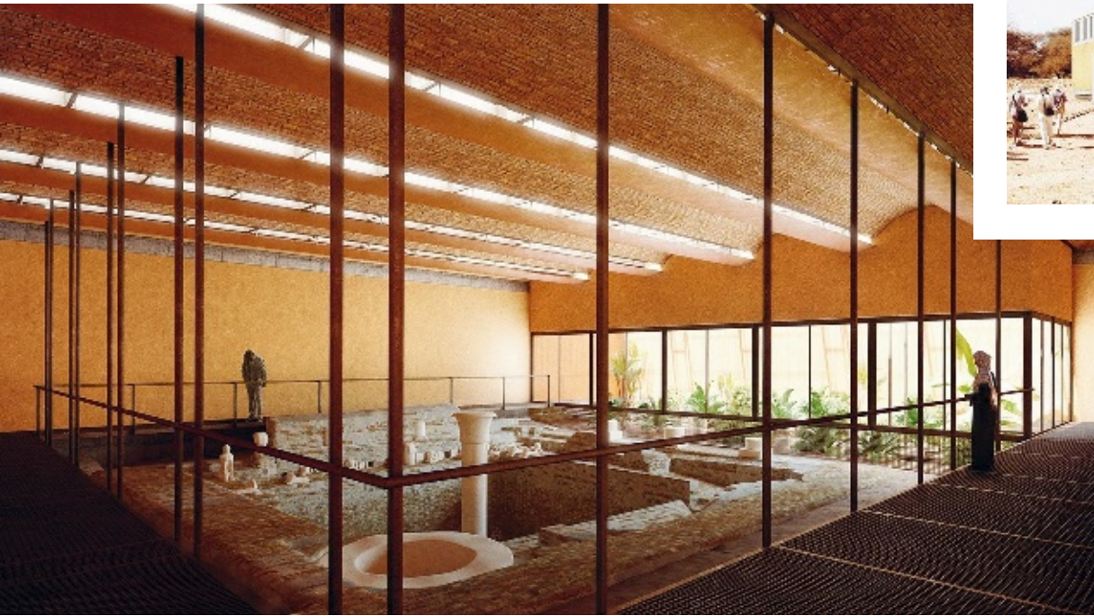
Two renderings of the Meroe Royal Baths Protective Shelter in Meroe, Sudan, an ancient city dating back to the first century AD and now listed as world heritage by UNESCO. The project provides a protective structure against wind and weather for the Royal Baths, and will be made with a thick wall of mud bricks to control internal humidity and natural ventilation.
